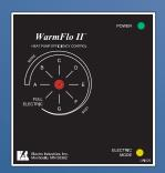
By adjusting the front panel efficiency dial you can determine how quickly you would like the WarmFlo to assist the air source heat pump. Choosing the more efficient settings increases the run time of the air source heat pump but decreases the temperature coming out of the duct registers. Choosing the less efficient setting decreases the air source heat pump run time but provides better warm air comfort coming from the registers.
